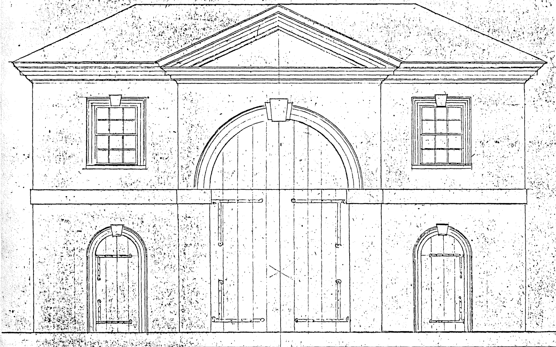
Fig. F-14. "Old Stable in Roxbury," measured drawing by Ogden Codman, Jr. (ca. 1890?). A typical Federal stable similar to Hunneman sketch from memory of Shirley-Eustis House stable (Fig. B-5). (Codman Collection of Architectural Drawings, SPNEA)
